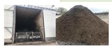
The process would involve reception of waste in a sealed negative pressure building, shredding and mixing of waste, then storage of waste in an enclosed composting tunnel before being transferred to an outdoor aerated static pile composting facility for stabilisation/maturation and then screening. Any unsuitable material would be sent off site to be re-processed into a biomass fuel for energy and/or heat recovery.
